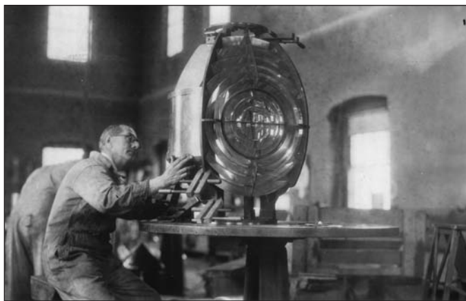
Lampists work to (top) repair glass in a lens, (middle) attach a sun valve to a lens, (bottom) fit a dark sector to a third-order lens. U.S. Lighthouse Service photos from 1930 courtesy of the U.S. Coast Guard.
