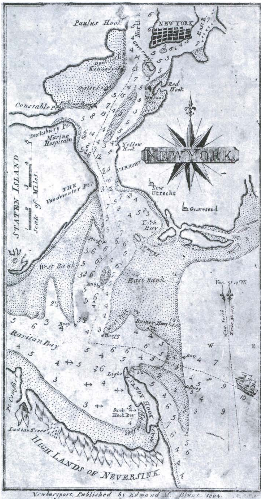
An 1804 chart of New York Bay. Sandy Hook Lighthouse can be seen in the lower center of the chart. The soundings of the depth of water are in fathoms. (One fathom equals six feet.) Notice that there are two buoys depicting the entrance to the bay and a few more to guide the mariner into New York City.
