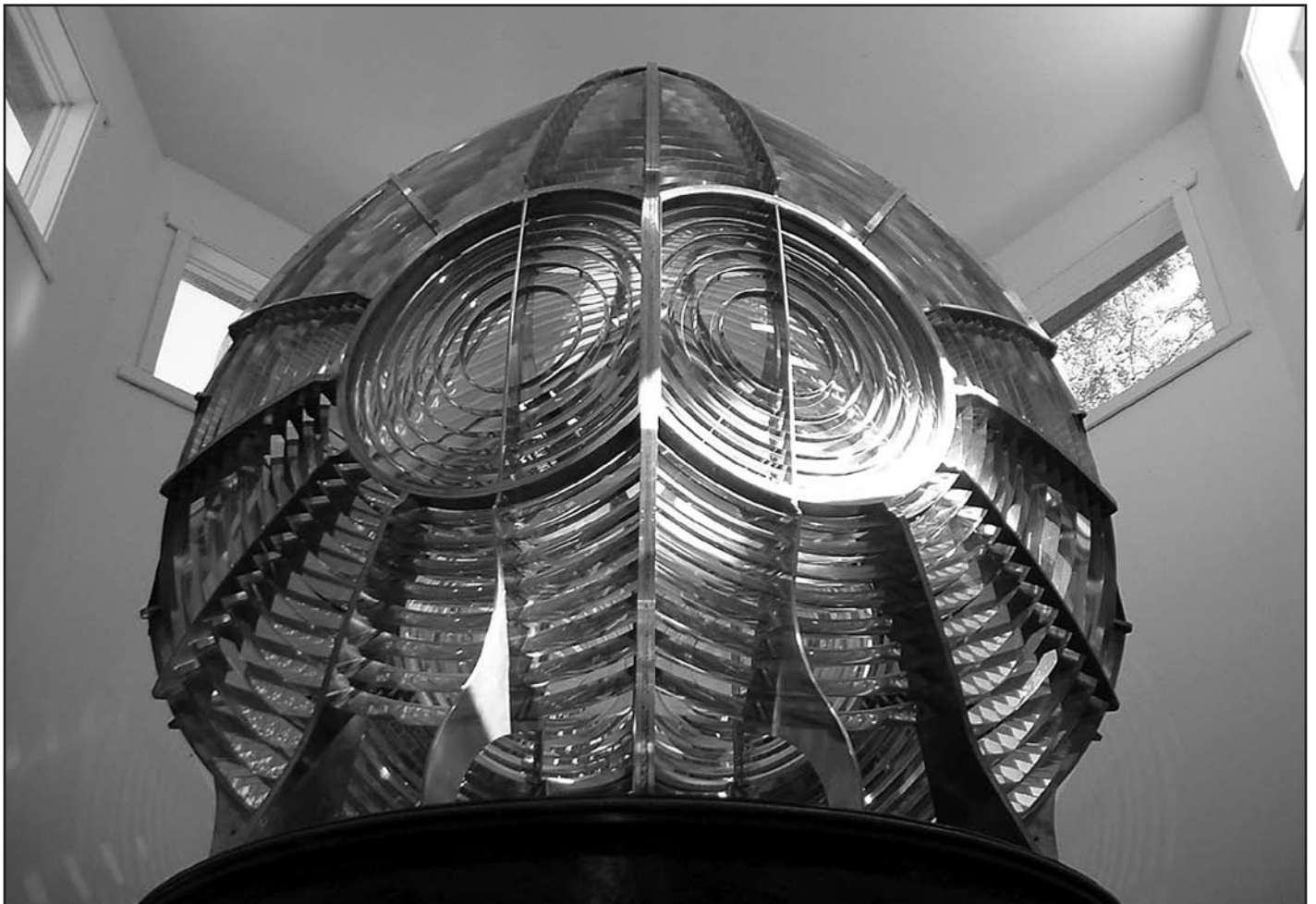
The Rock of Ages 2nd order Fresnel lens in the Windigo Visitor Center at Isle Royale National Park. The lens produced two flashes (group flashing white) every 10 seconds. 2002 photo by Eric Maul.
