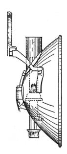
An Argand-type reflector initially used in the New Point Comfort lantern room. U. S. Lighthouse Society photo.
