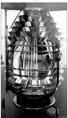
A fourth order Fresnel lens, similar to the one pictured, replaced the reflector system at New Point Comfort. U. S. Lighthouse Society
