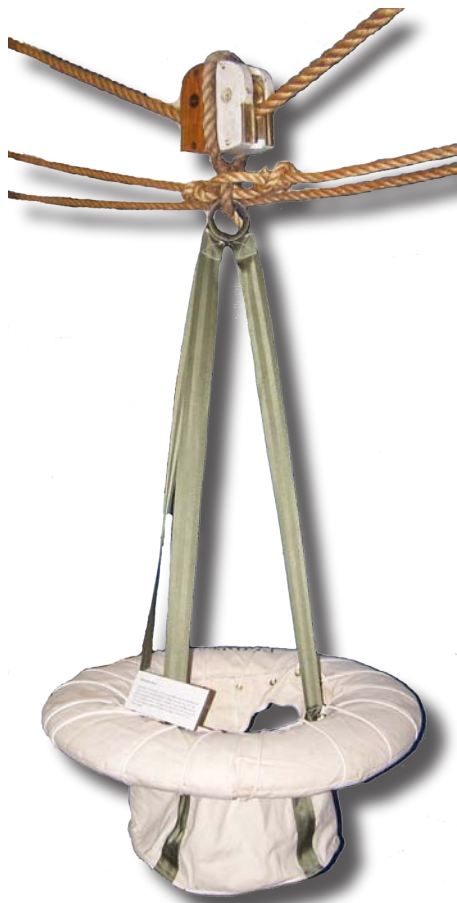
Breeches buoy on display at the Michigan Maritime Museum. USLHS archive photo.
