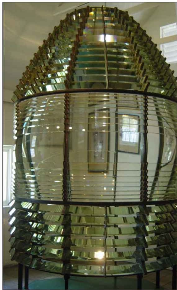
First-order Fresnel lens from Sombrero Key, on display at the Key West Lighthouse Museum. USLHS archive photo.
