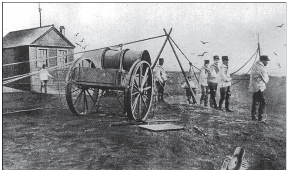
A beach cart in use during a line throwing drill. Note the Lyle gun lower right. USLHS archive photo.
